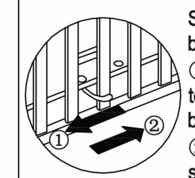
Secure the mattress board to front rail: ).Push handle to left to release mattress
