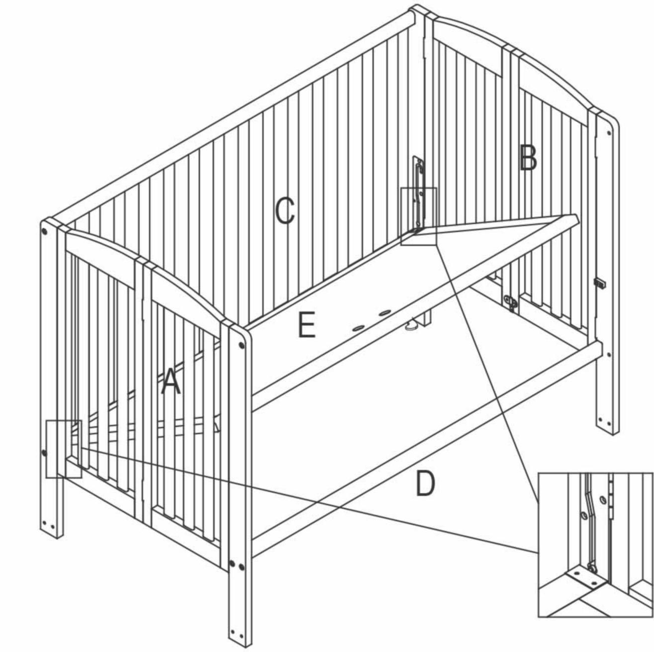
require height of the 2 level.slide in the bolt underneath the mattress board(E) to keep the mattress support fixed.
